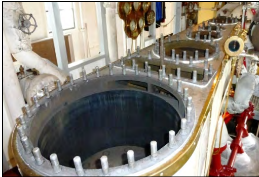
Virginia V's Triple-Expansion Double-Acting Reciprocating steam engine. Cylinder bores are: 10 1/2 inches, 16 3/4 inches, and 28.5 inches.
